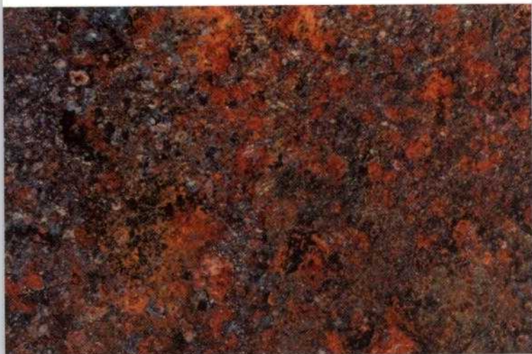
INITIAL CONDITION D
